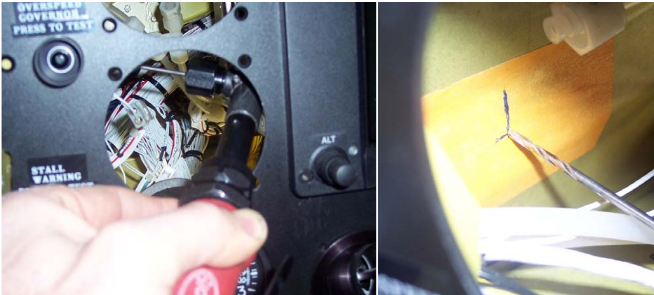
Figure 5-7: Drilling Pilot Hole for Lower Windshield Screw
