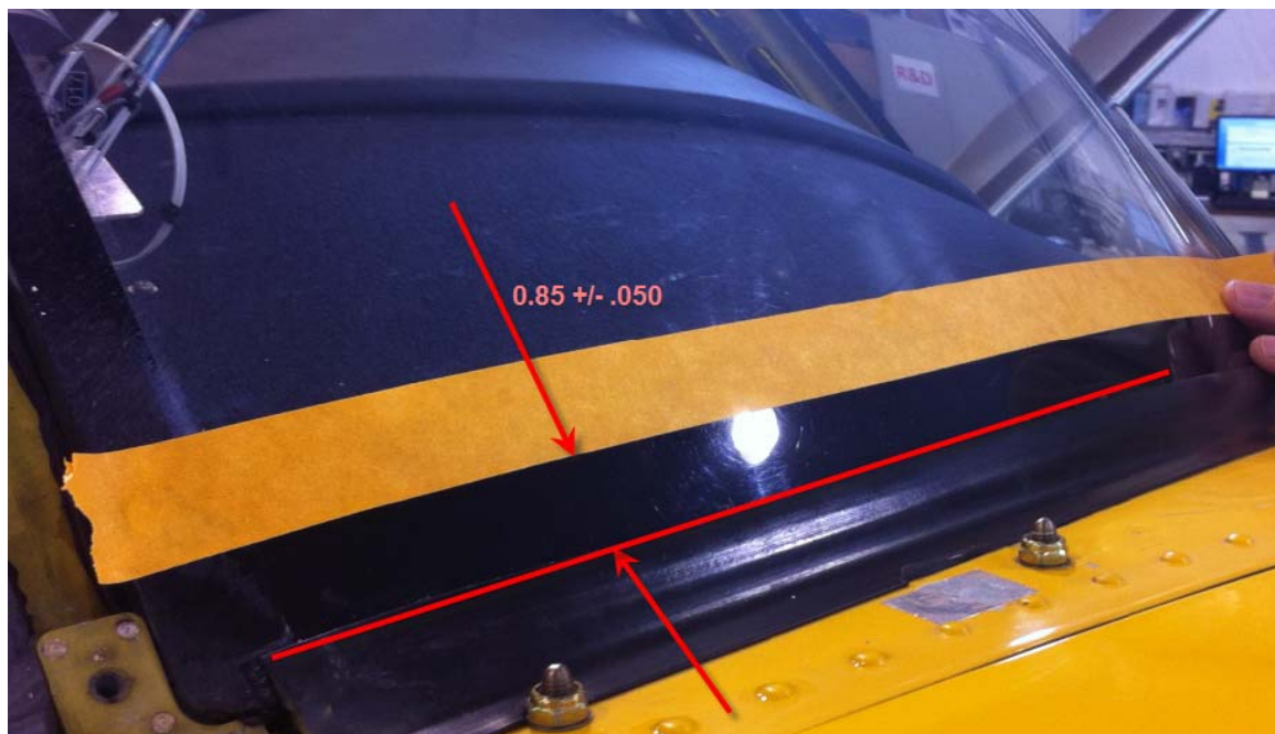
Figure 5-12: Masking Off 0.85" Measurement
