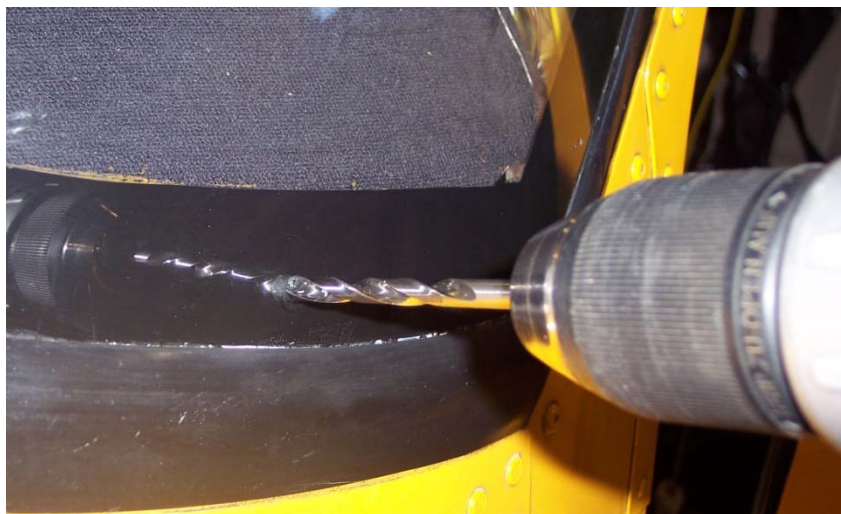
Figure 5-8: Drilling Through the Windshield and Boot Cowl
