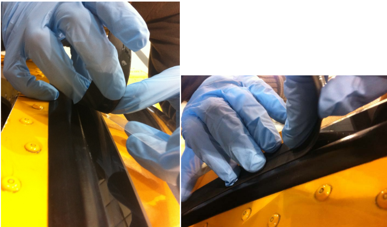
Figure 5-13: Installing the New Windshield Stripping
