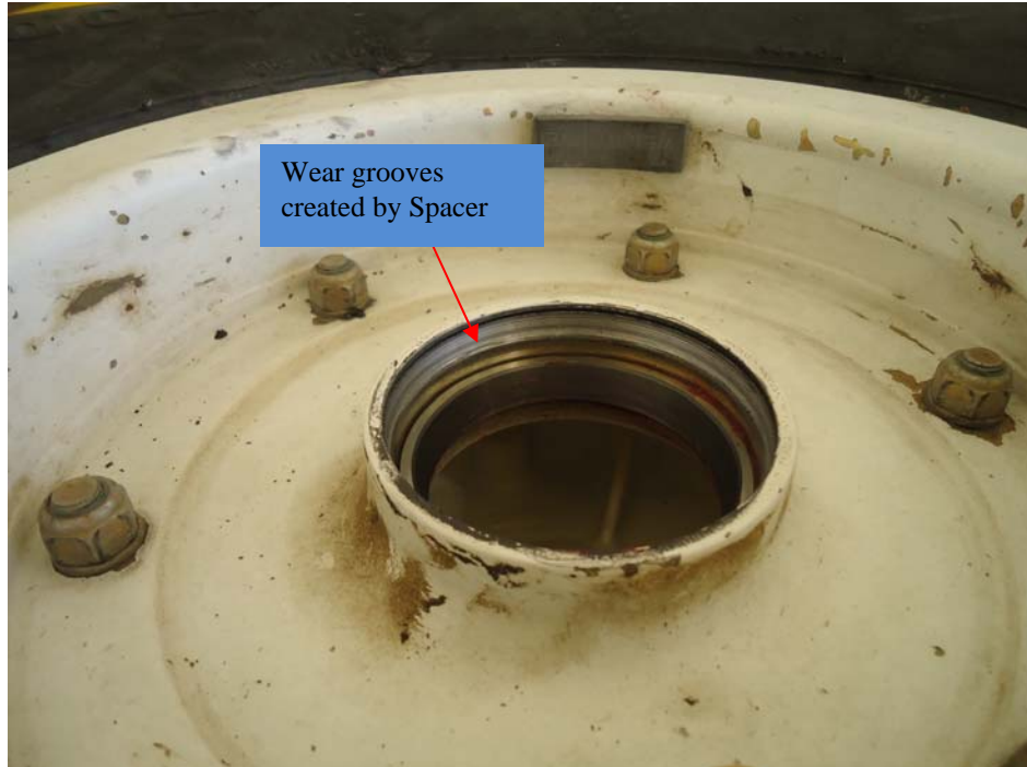
Figure 5-1: Damage to Grease Seal Bore
