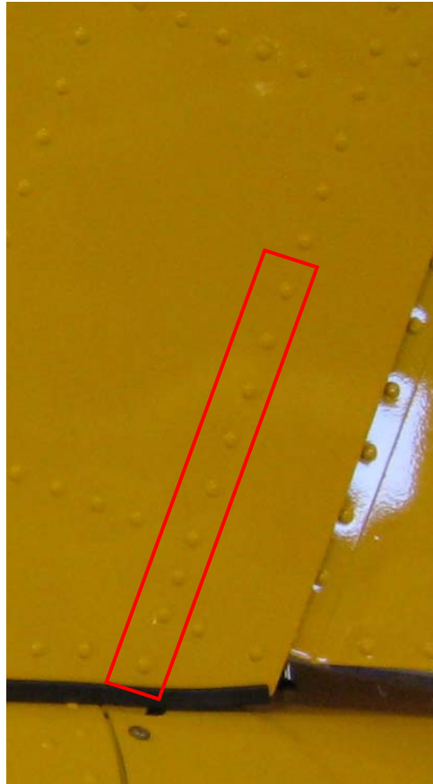
Figure 5-12: Aft Spar Rivets to be Replaced
