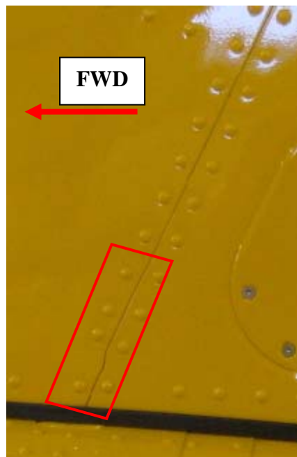
Figure 5-11: Forward Spar Rivets to be Replaced
