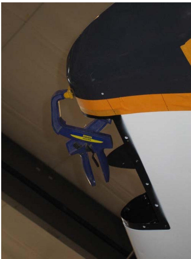
Figure 5-5: Clamp the Wingtip
