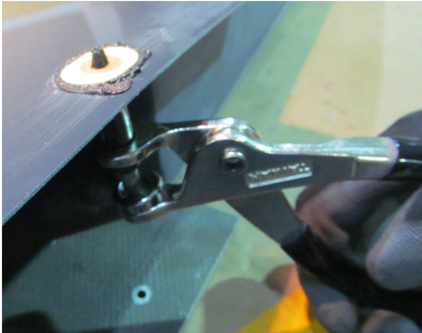
Figure 5-14: Installed Bonding Washer
