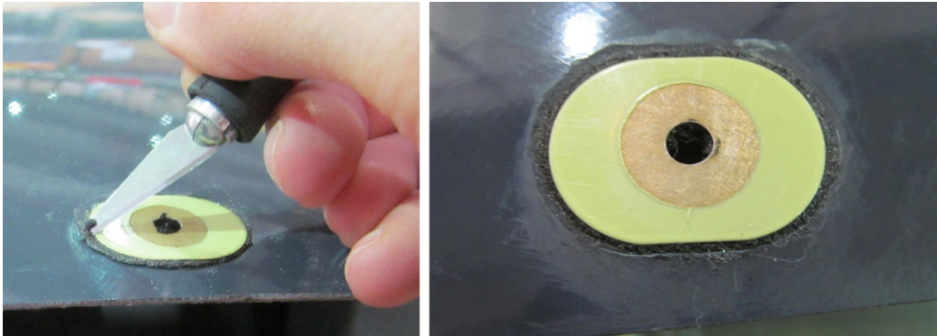
Figure 5-18: Remove Excess Cured Sealant
