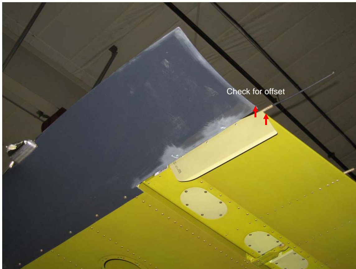
Figure 5-6: Check Aileron/Wingtip Alignment
