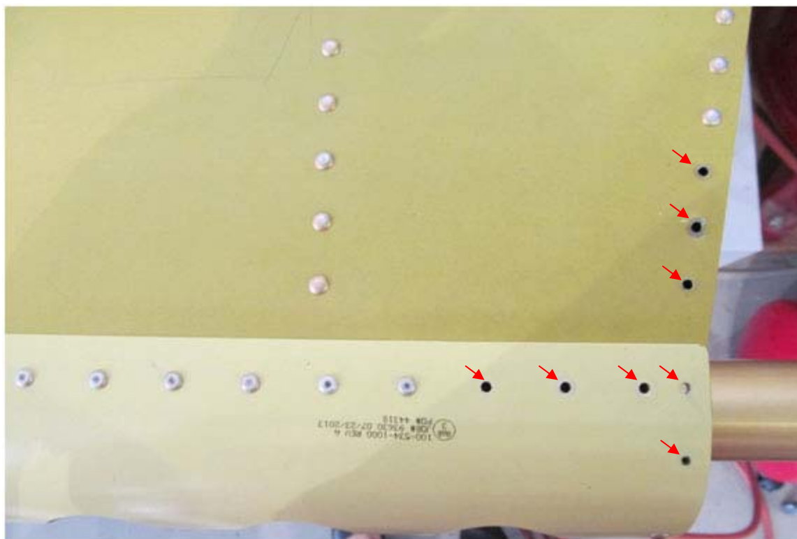
Figure 5-1: Drill Out Eight Rivets
