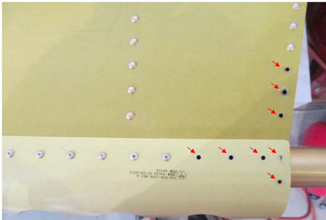
Figure 5-5: Drill Out Eight Rivets
