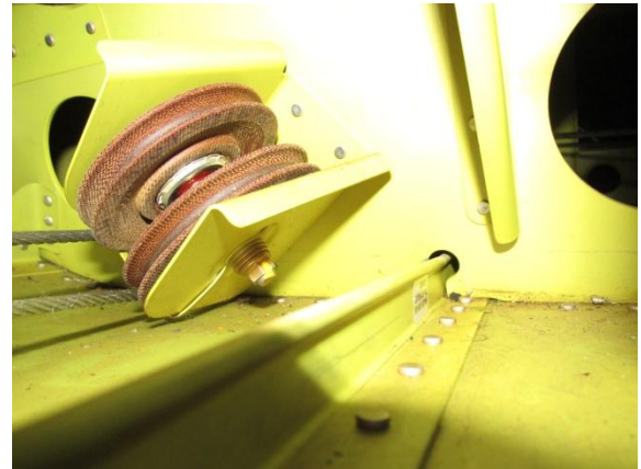
Figure 5-3: Pulley Bracket Viewed From Aft Looking Forward
