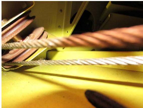
Figure 5-3: Pulley Bracket Viewed From Aft Looking Forward
