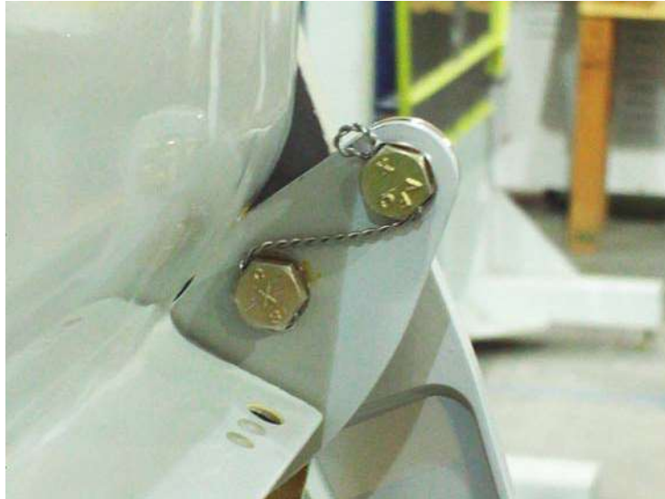
Figure 5-3: Safety Wire Installation
