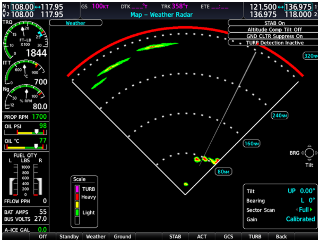
Figure 7-13. Weather Radar Screen
