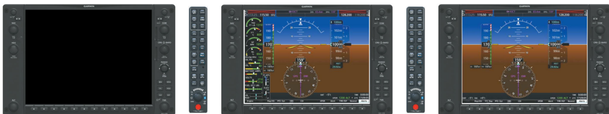
Figure 2-11. Reversionary Mode (Failed PFD)
